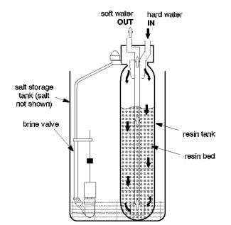
1 FILL: Salt, dissolved in water, is called brine. Brine is needed to clean the hardness minerals from the resin beads. To make the brine, water flows into the salt storage area during the fill stage as shown in FIG. 6. Fill cycle length depends on how much soft water making capacity you have used since the last regeneration. As you use more water, fill time increases so more brine is made. The greater amount of brine cleans more hardness minerals from the resin bed.
